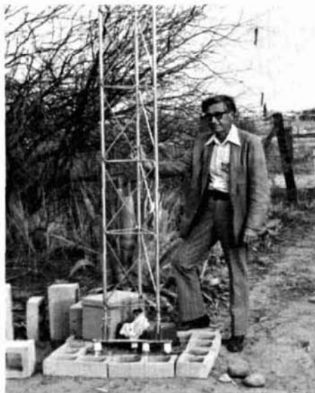
Author W7IV supporting W7IR's antenna. Concrete base is 18 inches (45.7cm) by 1 foot (30.5cm). Tuning network and ceramic insulators are shown.
